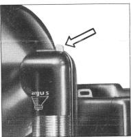
Best results will be obtained if General Electric "SM" or Sylvania (Wabash) "SF" flash bulbs are used. Any shutter speed may be used with either of these flash bulbs. When more light is necessary, midget base wire-filled flash bulbs may be used with the shutter at 25 (1/25) only. As a reminder, the figure 25 is colored green.
